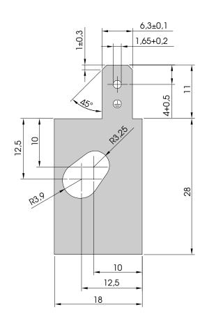
Werkstoff: Stahlblech 0.8 ± 0,03, vernickelt / Steel nickel-plated / acier nickelées
